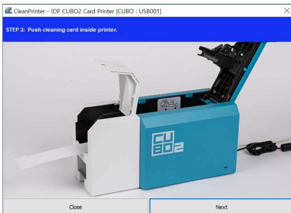
Figure 98 Printer cleaning Step 3
