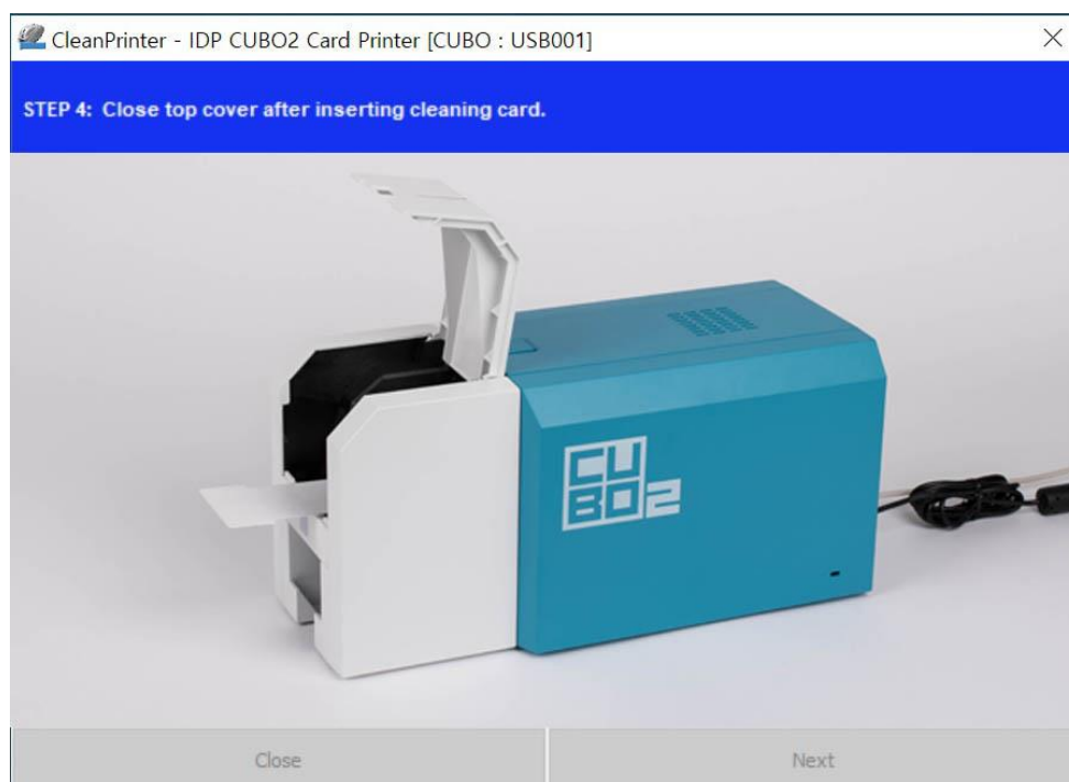
Figure 99 Printer cleaning Step 4
