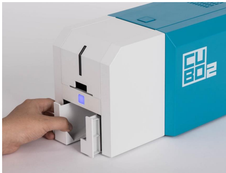
Figure 27 CUBO2 Dividing a stacker
