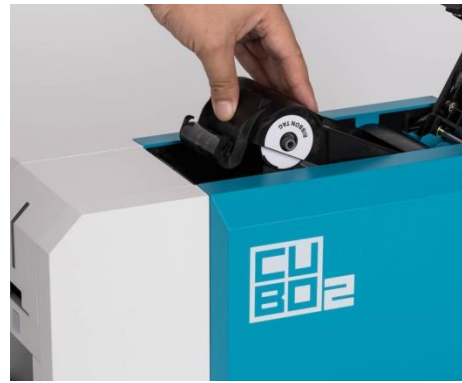
Figure 17 Installing the ribbon cartridge
